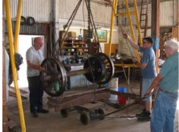
Andrew Gilbertson, Mike Crabb and Ian Seymour have just rolled the last wheel to be turned for Ballarat's tram 38 from the lathe shed to the workshop on 26 February 2010. The channel behind Ian is used as a rail track for the trolley to run in between both sheds.
