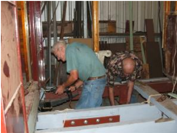
Michael Crabb & Bruce Lock working on the air brake assembly on 'Bib & Bub' tram 14 on Friday 26 February 2010.
