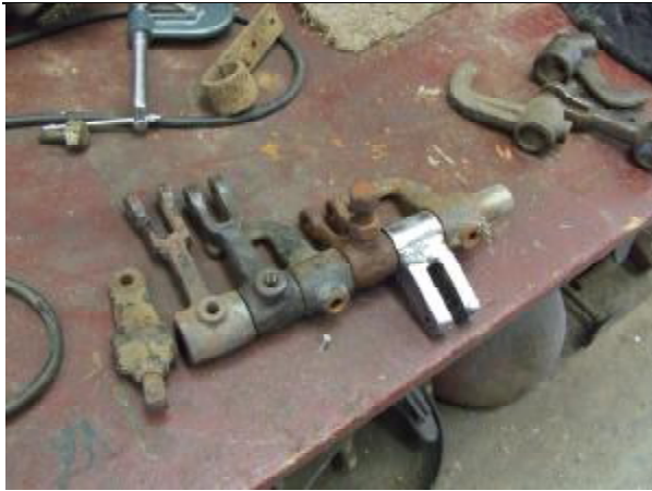
A mix of old and new; one of the new lifeguard components fabricated by Bruce Lock alongside original cast components.
