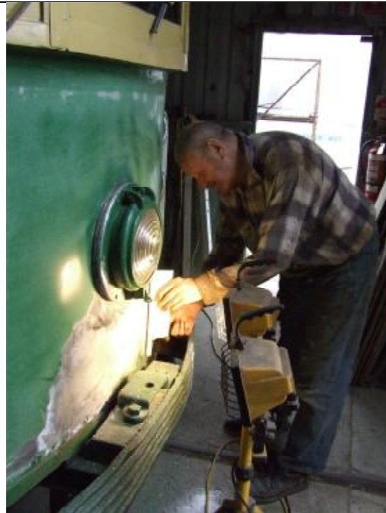
Bruce Lock resurfacing the end of W7 1013 after knocking out the worst of a bad dent that existed in the apron from its days in Melbourne.
