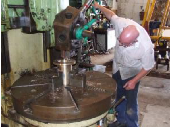
Ian Seymour machining one of the motor suspension bearings for Ballarat Tramway Museum's No. 38. Kym Smith
