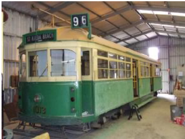
W7 1013 in the Bodyshop, with the saloon side panels on the northern side already sanded back for repainting.
