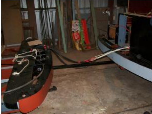
The simple but effective coupling arrangement between trams 14 and 15 as seen on 25 July Ian Seymour
