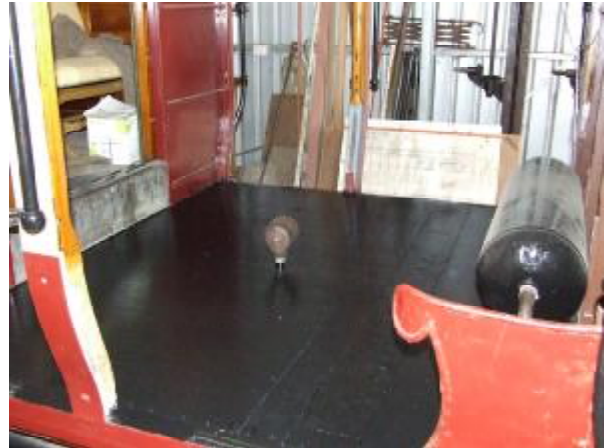
The air inlet filter and the air reservoir are the only easily visible parts of the air system now that the flooring has been installed in the drop ends of tram 15.
