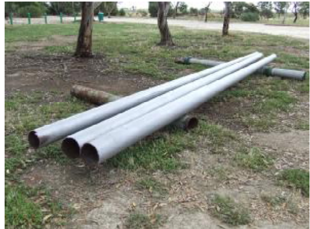
Here's three we prepared earlier! Three full length poles that have been prepared for future use, most likely as replacements for Poles 31N and 34N at the Mangrove Street Loop, and Pole 49 at the Playground Terminus.
