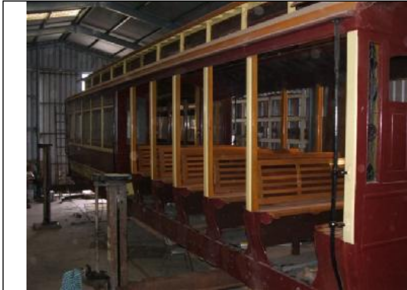
The recently installed crossbench seats in 'E' car 118 now give the tram its half saloon and half open combination appearance. Chris Summers 01 AETM Aug
