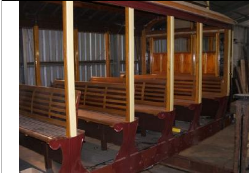
Another view of the recently installed crossbench seats in 'E' car 118. Chris Summers 02 AETM Aug
