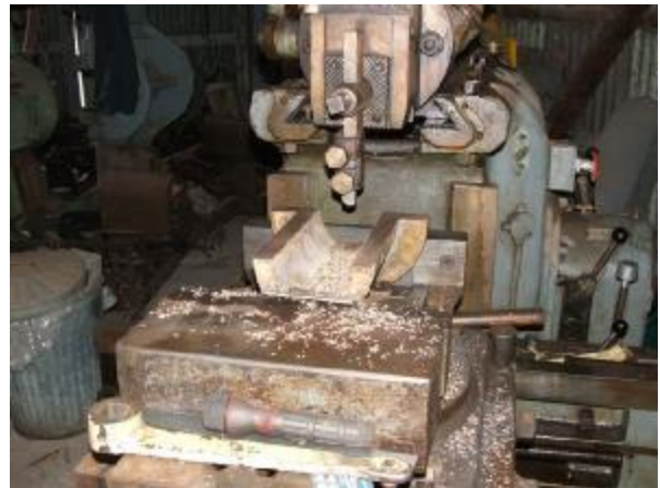
Machining of motor suspension bearings for 118. Machining joining surface square to faced off end surface. Chris Summers.
