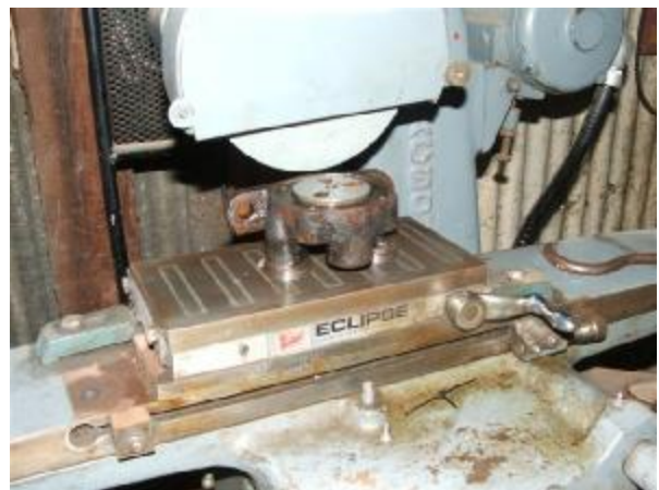
Grinding SL1 Brake Valve for tram 118. Chris Summers.
