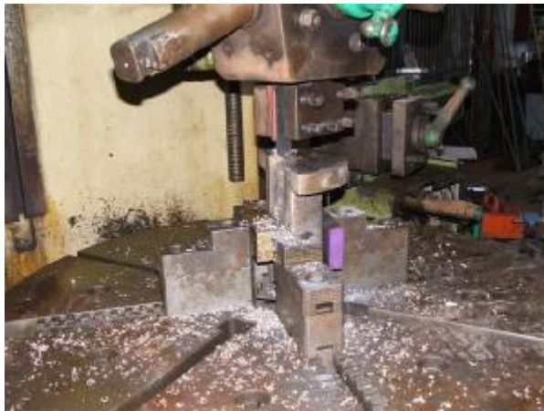
Facing off end one half of motor suspension bearing for 118. Chris Summers.
