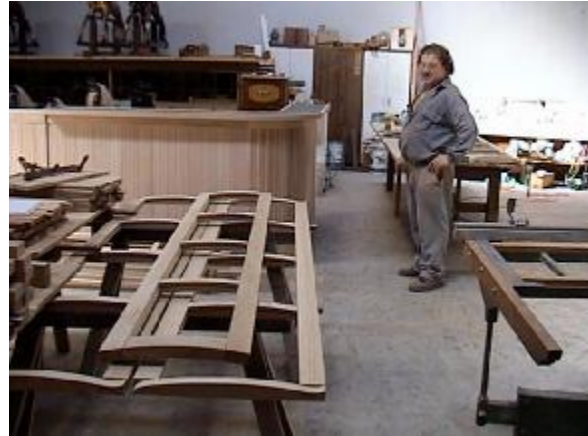
Photo taken in December of Mirko Husnjak fabricating seat backs for A 14, A 15 & E 118 at his joinery
